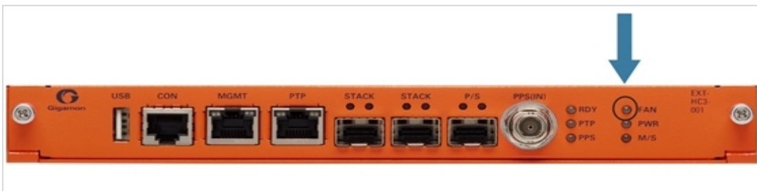
Figure 5: Global Fan LED Location on GigaVUE-HC3 Front
